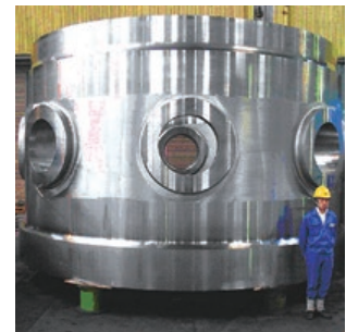
Shell flange used for pressure chamber for nuclear power plant
