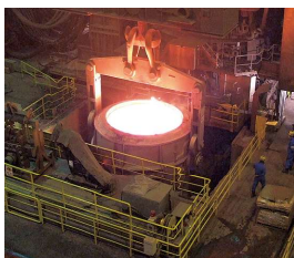
120トンハイパワー電気炉 High-Power 120-ton Electric Arc Furnace
